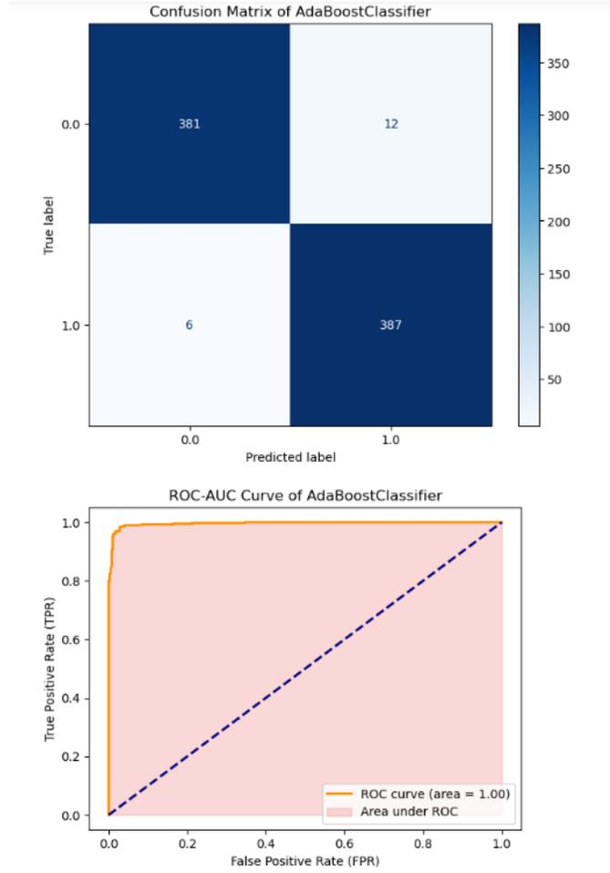
Fig4: Confusion matrix and ROC-AUC curve for Adaboost Classifier
