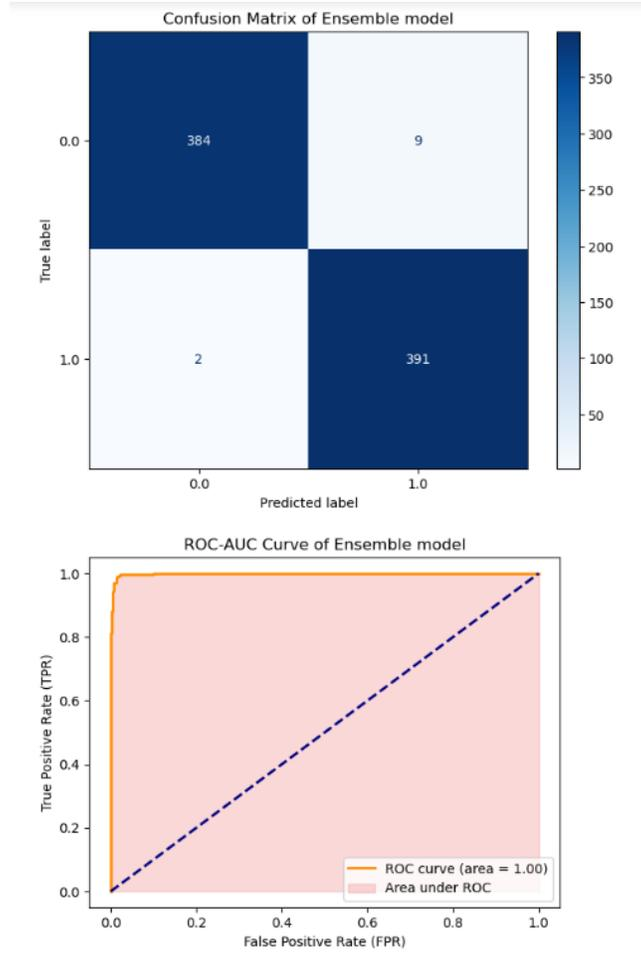
Fig6: Confusion matrix and ROC-AUC curve for Voting Classifier (Final ensemble model)
